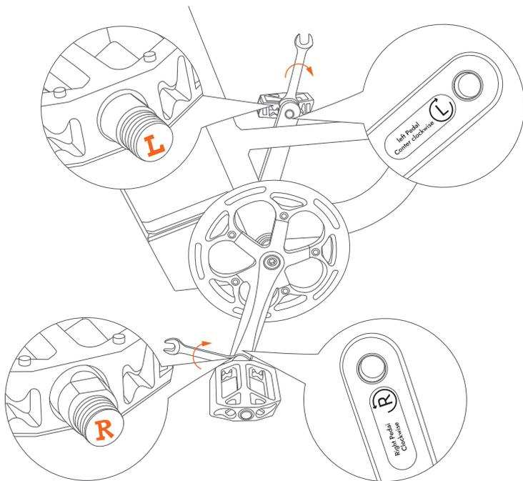
Use the open spanner of the tools bag, screw the pedal shaft into the threaded hole and tighten it in the direction of the arrow.
