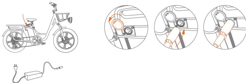
1. Charging connection: Connect the charging interface of the charger to the charging port, then connect the power plug of the charger to the power socket.
