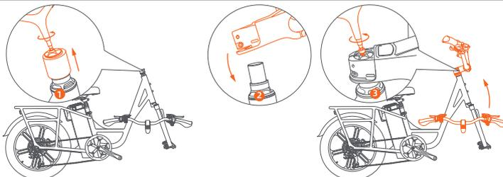
① Remove the protective sleeve from the fork riser: Use the hexagonal tool to unscrew the riser screw and remove the protective sleeve.
