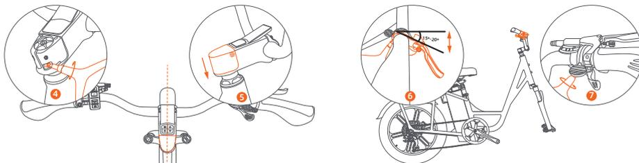
④ Adjust the bike front: Adjust the front of the bike like the above picture, align the stem with the front wheel, make sure they are in the same line and then lock the screw on the left and right sides of the handle in turn.
