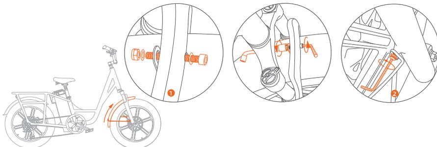
① Put the front fender through the gap of the tire and fork, then screw tightly.
