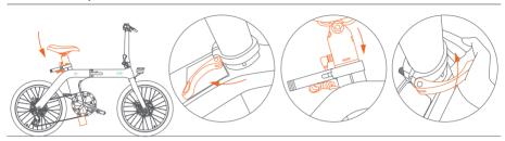
Lift the seat clamp upward, to keep it in open status. Gently press down the seatpost to the bottom. Press down the seat clamp to keep it in closed status.
