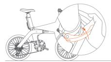
③ Buckle the seat clamp to ensure that the seatpost battery won't slide down
