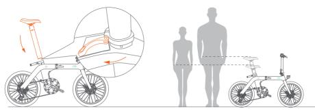
① Open the seat clamp, insert the seatpost battery.
