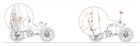
$\ensuremath{\textcircled{\textcircled{\scriptsize 1}}}$  Open the quick release, adjust the handlebar direction upward to loose the wire.
