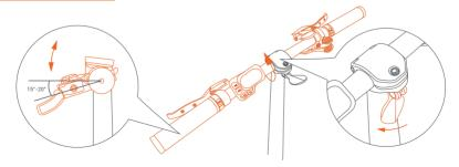
③ Adjust the handlebar direction, to make it at an angle of 15°-20° with the horizontal line, then close the quick release, to complete the unfolding stem.
